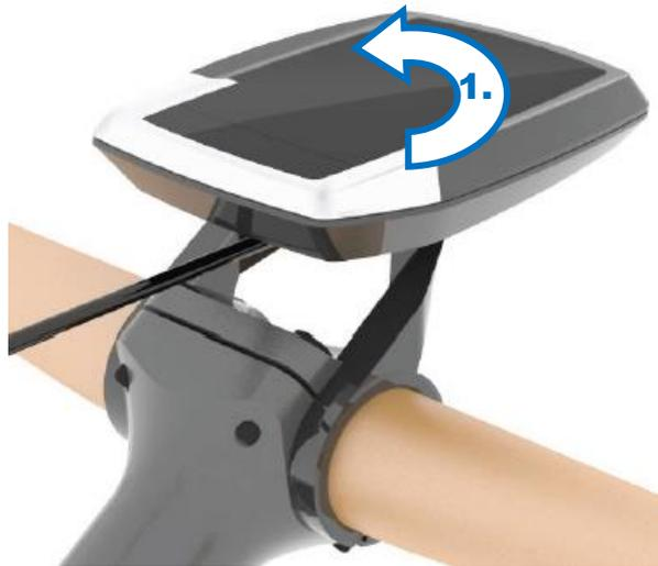
Fig. 7: releasing the display
