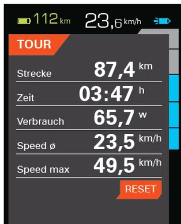
On the site TOUR information about trip distance since the last RESET are shown. These data are cumulated as long as the HMI is in operation.
