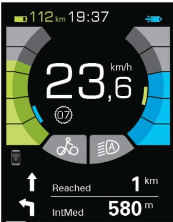
For displaying the navigation on the main display your smartphone has to be connected by the Naviki App (not included in delivery) to the system and an active route has to be in the App. Pay attention to the smartphone symbol below the battery's state of charge at the bottom left corner.
