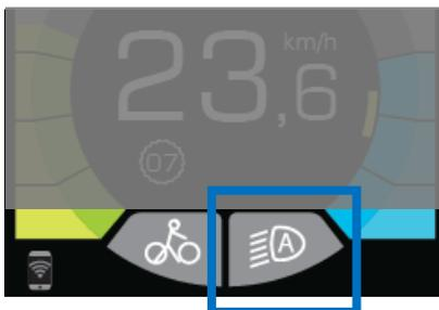
By switching on the system the low beam is activated generally. According to model and built-in lights button T8 can be pressed for 0,5s to change the light between high and low beam.
